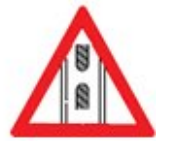
GAP IN MEDIAN
